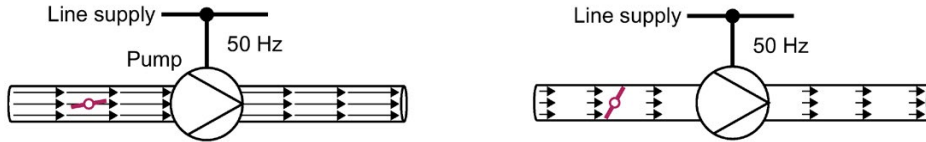
Figure 6-73 Flow control with pump and throttle connected to a 50 Hz line supply
